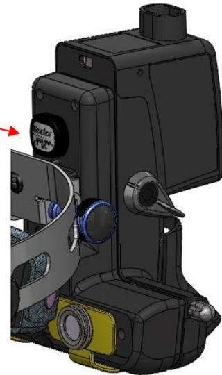
Note that the LION should only be used with the LION LED. Ensure that the red switch on the rheostat is in the direct shown in the figure below. The symbol shown on the rheostat indicates a bulb light source.
