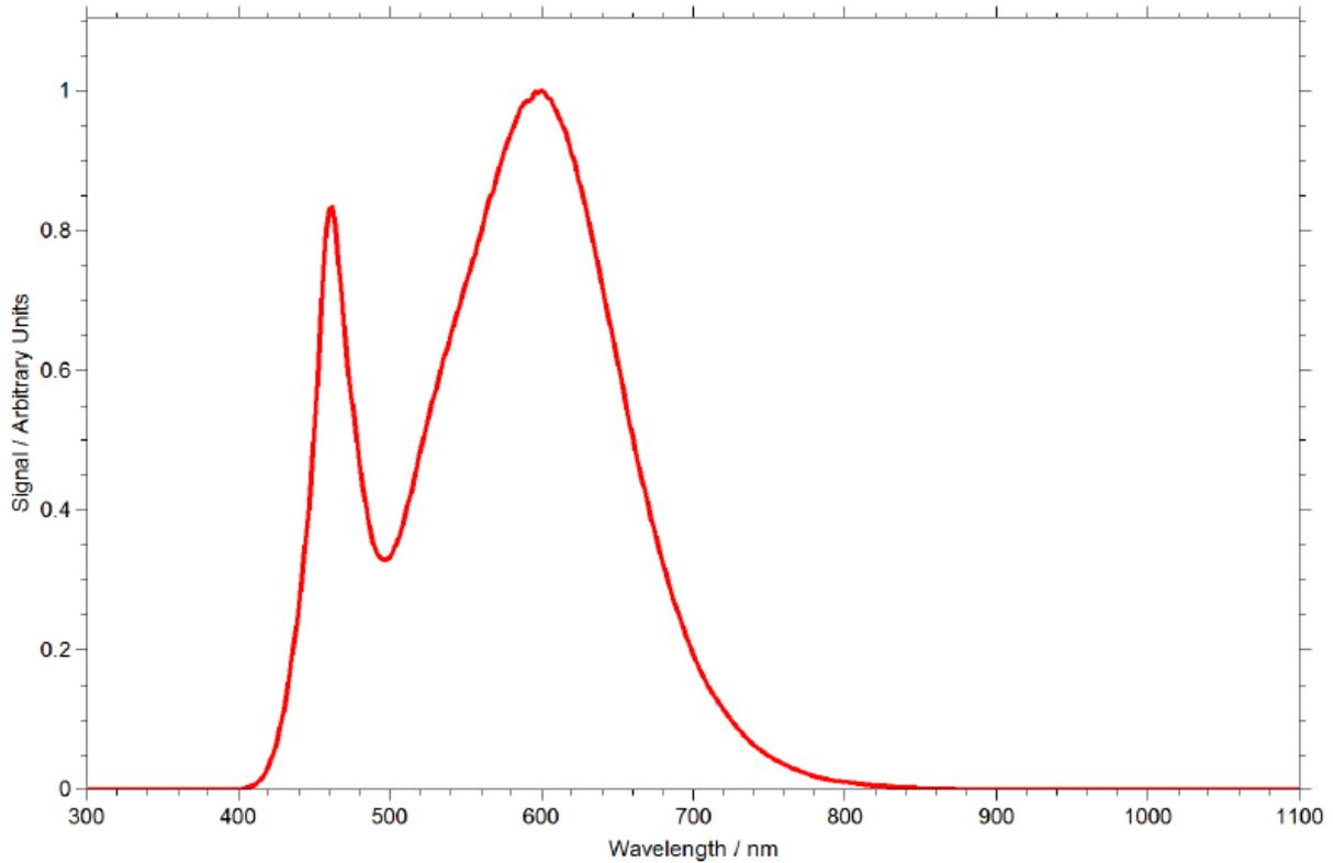
**Relative spectral output of LED light source**
