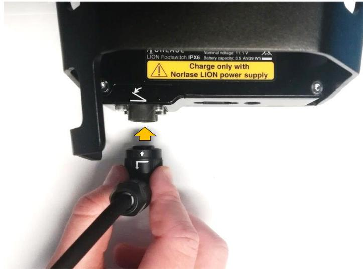
2. Push connector into the foot switch receptacle until it “clicks” and locks into place
