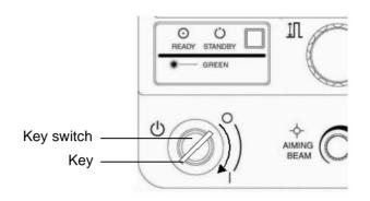
When the main body is activated, "Self Test..." is shown on the Status display window and the self-check function works, turning on display windows in order.
