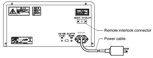
Remote interlock connector.. Connects the remote interlock switch. Power cable
