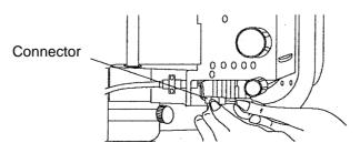
**3** Turn the Lamp holder knob, remove the illumination lamp together with the socket, and then pull off the lamp.
