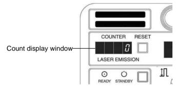
Even when the Emission switch is released in the middle of emission, it is counted as one emission count.
