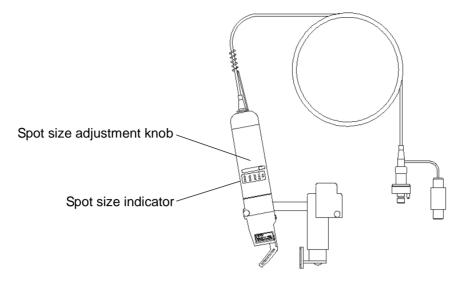
If the aiming beam is not in focus, the spot size (coagulation spot) does not follow the display.
