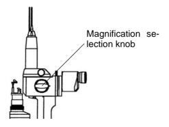
The magnification of observation can be selected in 5 steps by turning the Magnification selection knob. Select the total magnification for observation according to the indication around the knob.
