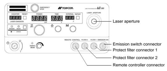
Laser aperture .......Plug in the laser beam fiber here. Emission switch connector ......Plug in the Emission switch or the Footswitch. Protect filter connector 1 ......Plug in the protect filter. Protect filter connector 2 ......Plug in the protect filter. Remote controller connector .....Plug in the remote controller.
