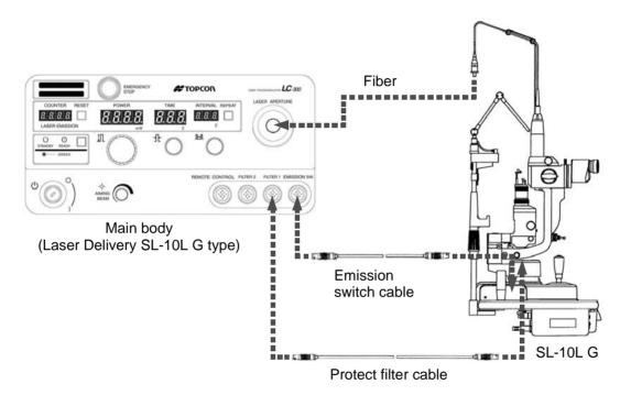
For connection with LC-300G, necessary cables are attached to SL-10L G as standard accessories:
