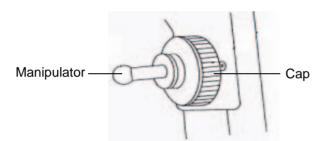
**1** To release the manipulator, turn the cap counterclockwise.
