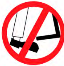
Figure 1-6. Foot entrapment hazard.
