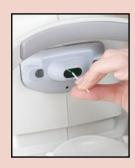
Moisten the Topcon q-tip with solution. Insert the q-tip into the nozzle. Lightly touch the glass surface while turning the q-tip. Replace the q-tip with a new one and wipe the surface in a similar fashion. Cleaning is completed when the grease is thoroughly removed and the fixation target is clearly seen.
